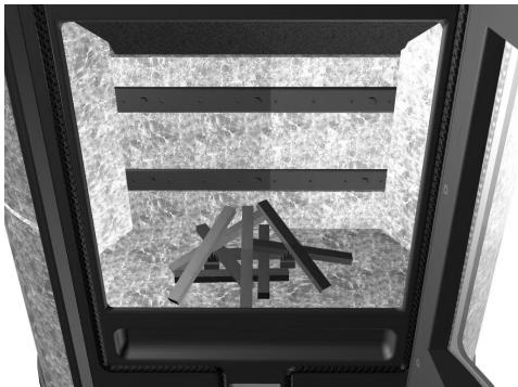
Position firelighters in the middle of the hearth. Build a pyramid of kindling around the firelighters. Light the firelighters. Choosing the right kindling (size and type) allows heat to be generated more quickly. Preferably use finely chopped lightwood. The faster the stove reaches maximum temperature, the faster circulation is established, and the less soot and creosote is created. This keeps the stove, smoke guide and environment clean.
