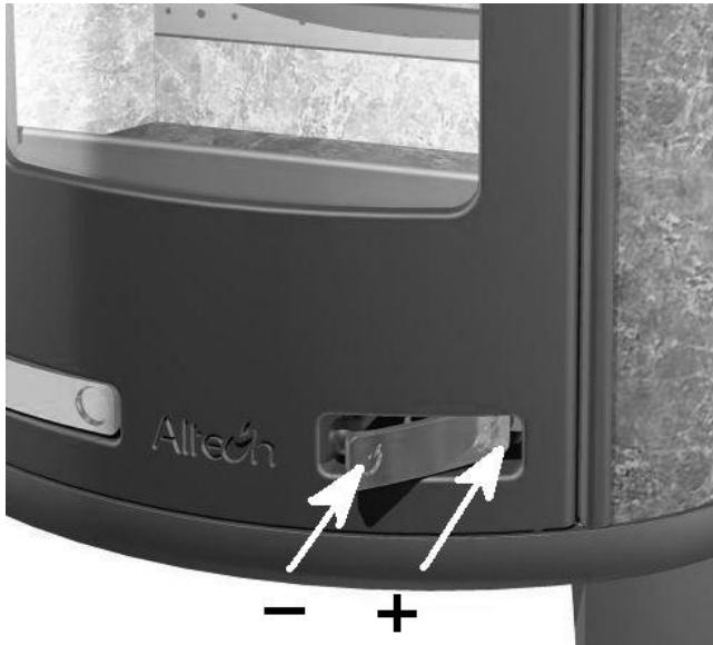
Once the fire has gone out completely and no embers are visible in the stove, close the air valve completely. The stove will then continue to give off heat for a longer period. When starting a new heating cycle, reopen the air valve
