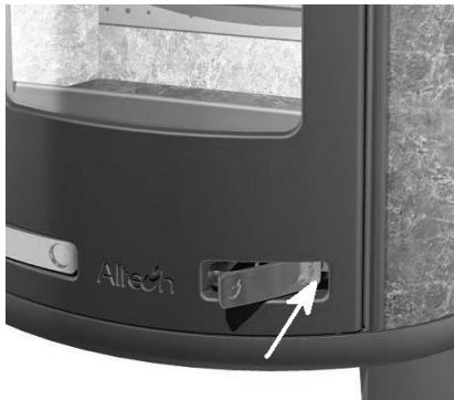
Remove excess (not all) ashes. NB, there can still be glowing embers after more than 24 hours after initial lighting. Always empty ash remains into a fireproof container.
