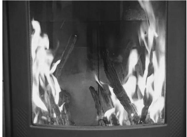
Close the door once the fire is burning well, this ensures a higher efficiency
